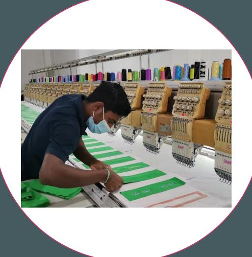
"We are equipped with two 20 — head and two 15 head embroidery SWF Embroidery machines, Laser- cutting machine, Needle detector with round the clock working capacity.
